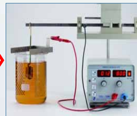
Rhodium plating Umicore RHODUNA® electrolytes according to operating instructions
