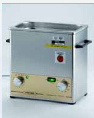
Ultrasonic degreasing (essential for polished parts) e.g. Umicore Cleaner 6030 (3-5 g/l)
