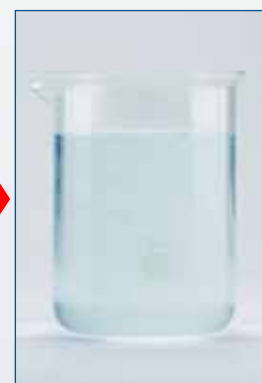
Acid dip 5% H 2 SO 4 solution, room temperature, 20-30 seconds
