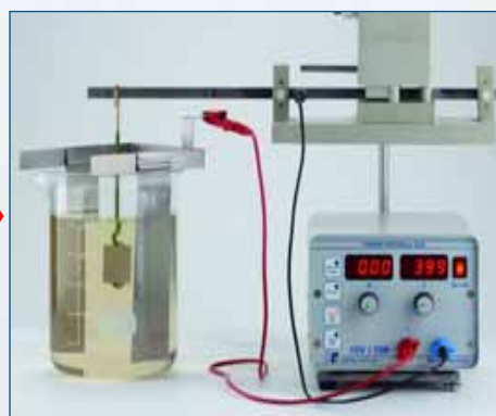
Cathodic degreasing (essential for all parts) e.g. Umicore Cleaner 6030 according to operating instructions
